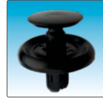
6985 Engine Under Cover & Push-Type Retainer; 90467-07201 Head Diameter: 20mm, Stem Length: 10mm, Fits into 7mm Lexus ES300/330 and Toyota Avalon, Cam Kaldırma Tamir Parçası
