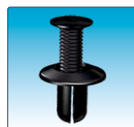
0264 Bumper Push-type Retainer, Black, HYUNDAI: 86590-28000; KIA: 0603250037A; Mazda: B092-51-833; Ford: MB-455-56143 Head Dia: 18mm, Stem Length: 12mm Fits Into 8mm Hole
