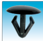
4144 Retaining Clip, Nissan 01553-00051 (HD: 18mm, Stem: 16 mm, snaps into 7 mm hole,
