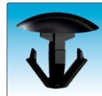
0461 Hood & Trunk Moulding Retainer Clip, Black, Replacement Honda & Acura 91518-SM4-003; Acura Integra & Honda Civic 1994 - On head Diameter: 12mm, Stem Length: 9 mm, Fits into 6mm Hole
