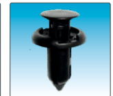
5728 Garnish Side Protector Push-Type Retainer, Honda: 90505-SX0-003 H.D: 18mm, S.L: 15mm (Not Including The Pin), Fits into 8mm Replaces Honda Odyssey 1995 - On CR-V '02-05 CR-V '06 CR-V '07-01 ODYSSEY '95-98 PRELUDE '97-01
