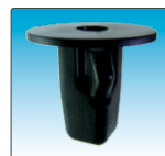
3244 Screw Grommet For Hood, (86848-22000) HYUNDAI , Lexus & Toyota : 90189-06013; Screw Grommet #14 (1/4") or M6.3-1.81 Screw Size HD: 20mm, S.Length: 17mm, Fits Into 8mm x 8mm Hole
