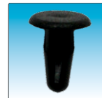
5623 Retaining Clip; Nissan: 01553-00291, Honda: 91518-S10-003 Mazda: 9926-40-543A Black Nylon Head Diameter: 11mm Stem Length: 15mm Fits Into 5.5mm Hole
