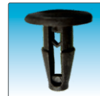
0498 WeatherStrip & Trim Panel Retainer, Brown, Replacement Toyota: 90467-07050; Honda: 90687-SA5-0030; Nissan: 01553-00172, Head Dia: 14,84 mm, Stem Length: 15, Fits: 7,5 mm
