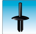
0014 Bumper, Wheel Opening, Scuff Plate & Interior Trim, Push-Type Retainer Head Diameter: 20mm Stem Length: 15mm Fits into 6.3mm Hole BMW: 51-11-1-944-537; Series 3, 5, 7 & X5 1989 - On
