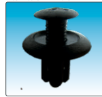
0601 Push-Type Retainer; Hyundai: 0G03250037A; Mazda: B092-51-833; Ford: MB-455-56143; H.Dia: 18mm S.Length:12mm Fits Into 8mm Hole
