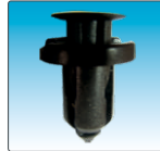
0011 Bumper Push Type Retainer, Nissan: 01553-09241 Head Dia: 18, Stem L: 15, Fits into: 10 mm
