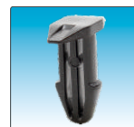
8199 Cowl Vent Retaining Clip, Black Nylon Head Diameter: 6mm x 16mm, Stem Length: 14mm, Fits Into 6mm Hole Replaces Acura & Honda: 91502-S84-A11 CL 2001-03, MDX 2001-06,
