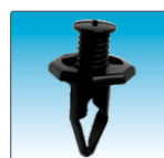
5467 Honda Bumper Fascia Push-Type Retainer H.D: 20mm, Stem L.: 24mm, Fits Into 10mm Replaces: Honda 91504-SM4-000 Accord 1990-On
