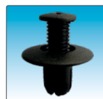
0267 Push-Type Retainer, Black, Long, MAZDA: FB01-56-964, Nissan: 63076-8596; Honda: 90675-SB3-003 => Replaced 90675-SB0-003; Head Dia: 20mm, Stem Length: 11 mm, Fits Into 8mm Hole ACCORD, CIVIC, CRX, PRELUDE
