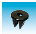
4796 Clip Screw, Black, (86848-22000) HYUNDAI , #10 Screw Size, Head Diameter: 17mm, Fits Into 9mm x 9mm Hole
